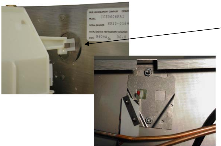
Proper position of wire bale switch actuator (Early 48 inch units)
