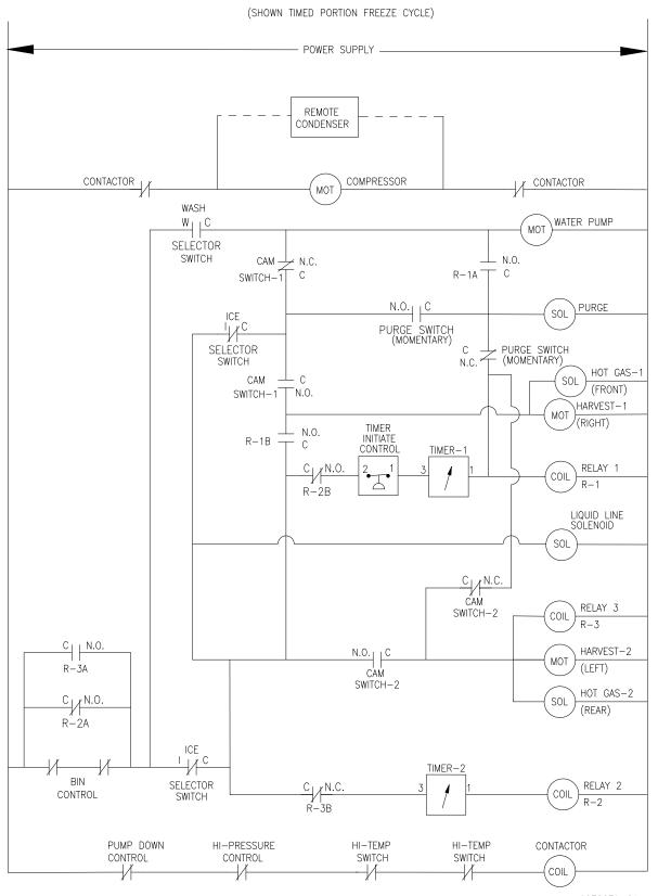
WIRING SCHEMATIC REMOTE COOLED
