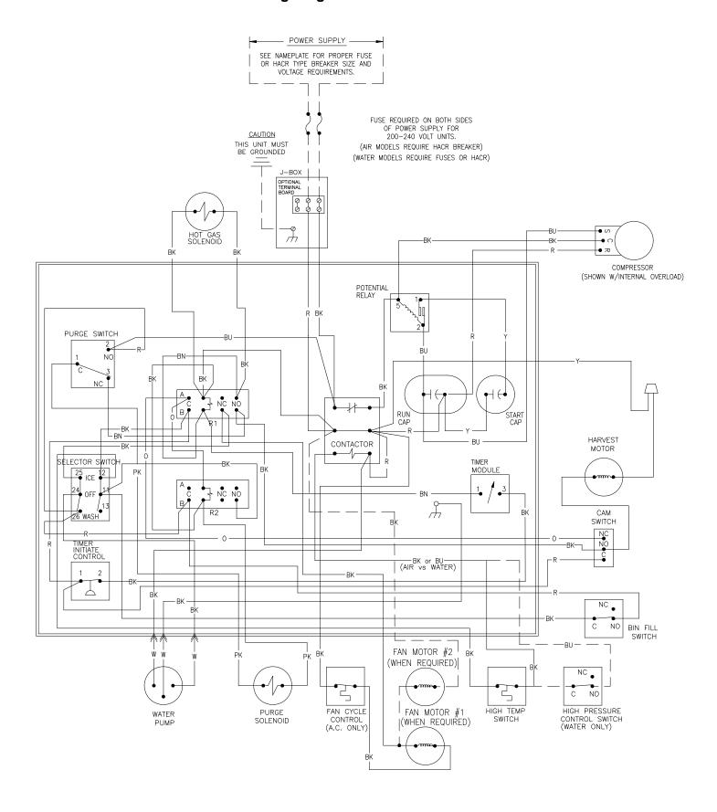
ICE Series Wiring Diagram
