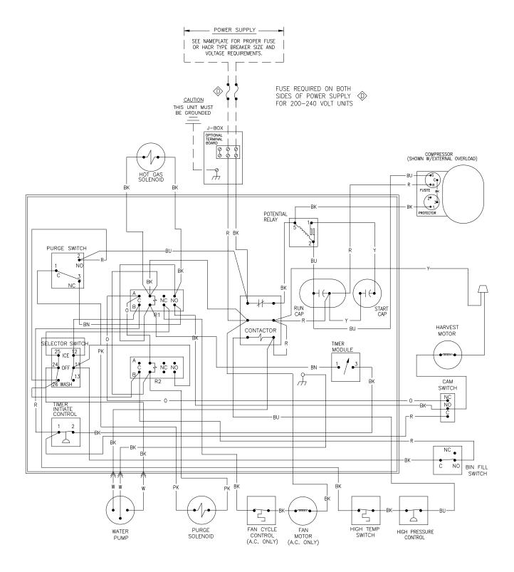
ICE Series Wiring Diagram
