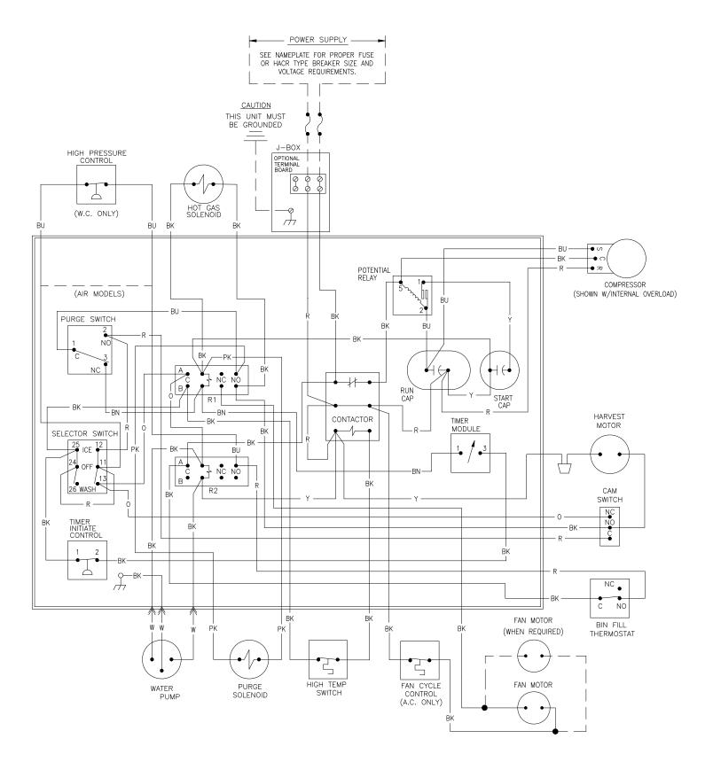
ICE Series Wiring Diagram
