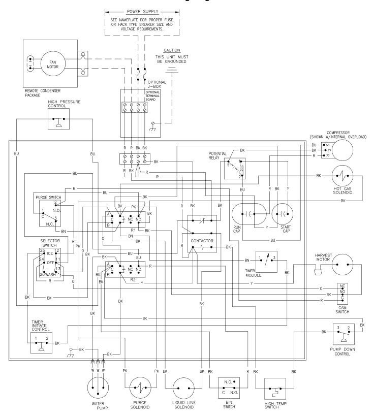
ICE Series Wiring Diagram
