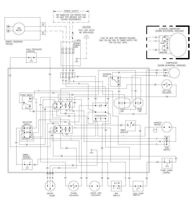
ICE Series Wiring Diagram
