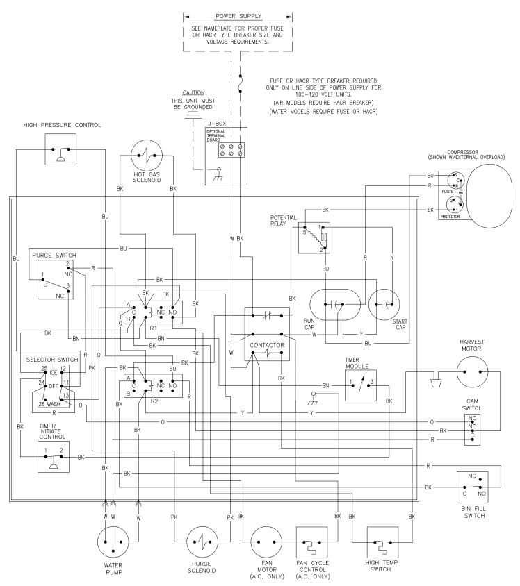
ICE Series Wiring Diagram
