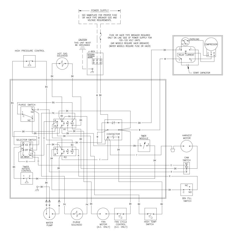
ICE Series Wiring Diagram
