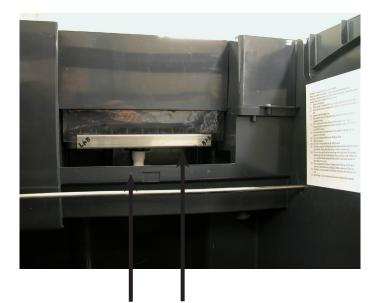
Front view of freezing compartment, shown without Ice Chute or Curtain. Right arrow points to Spray Platform, located under Ice Chute. Spray Platform inlet connects to pump hose and is snapped into clip at back of reservoir. Left arrow points to clip.
