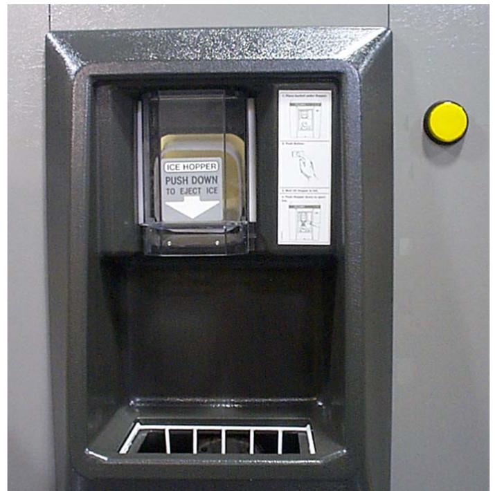
**Note: If the chute is not all the way up, the unit cannot resupply the chute with ice.**
