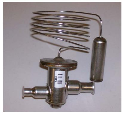
**Installation Note**: The new Danfoss TXV utilizes a stainless steel bulb. When installing a replacement Danfoss TXV valve, the bulb must be installed with the proper clamp and as tightly as possible to insure proper performance.
