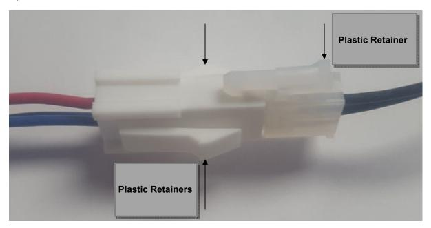
To separate the connectors, depress the two plastic retainers on the female portion of the connector while depressing the locking portion of the male connector; pull the two apart by separating the connectors, **DO NOT PULL** on the connector wires.
