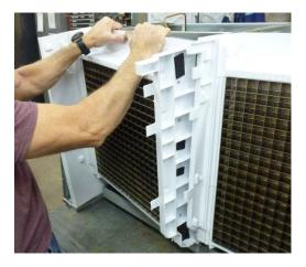
The new evaporator comes with two new side wall pieces. If replacing the left evaporator plate, you will use the right interior wall. If replacing the right evaporator plate you will use the right-side wall. These new pieces have cut outs to accept the updated evaporator plate.
