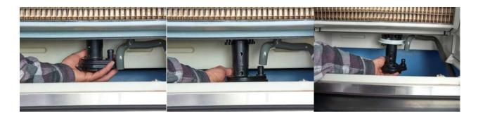
The "foot" of the Water Pump points towards the right front corner of the unit. Grasp the foot and turn counterclockwise. When the foot points towards the right rear corner, you will feel the weight of the pump as the collar clears the base connections. Lower the Water Pump and disconnect. Reinstall the Water Pump by first making the electrical connection, the push Pump up pointing the Foot at the right rear corner and turn clockwise to secure.
