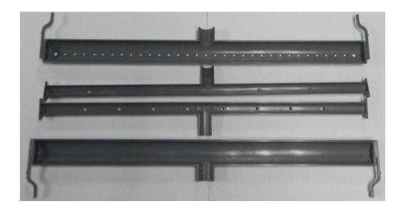
The Water Distribution Tube comes apart easily. It should be taken apart and cleaned regularly along with the rest of the unit. The pieces are Poka-yoke, meaning it only goes back together one way.
