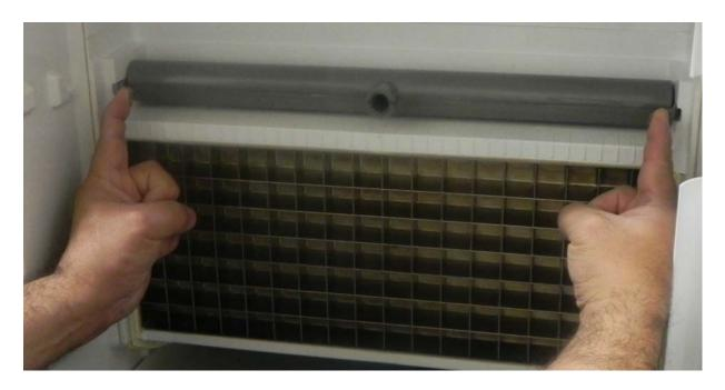
Gently squeeze the tabs inward on the Water Distribution Tube and forward towards the front of the unit.
