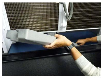
Installation of the sump is the reverse of removal. To ease the installation using one hand under the sump pan to lift on the back will help with the install. Ensure the left side is seated properly, before attempting to press the right side into place. *Improper placement of the left side can lead to damage of the retention features during installation.*
