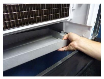
Next, lower the right side of the sump into the bin and release the left side of the sump.
