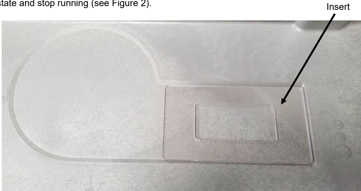
Figure 1: Sump insert shown in the proper position
