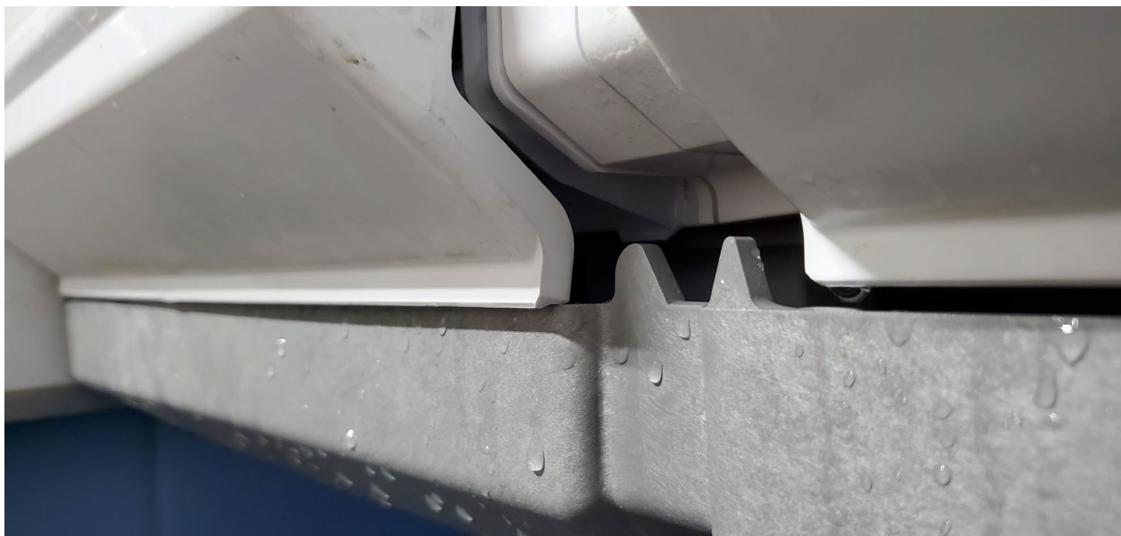
Figure 2: Interference between the sump and curtain when the insert is not installed
